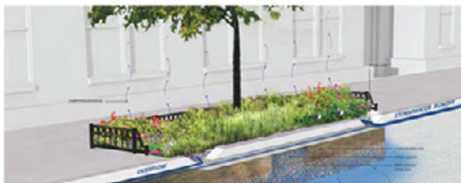
STORMWATER INFILTRATION TRENCH
