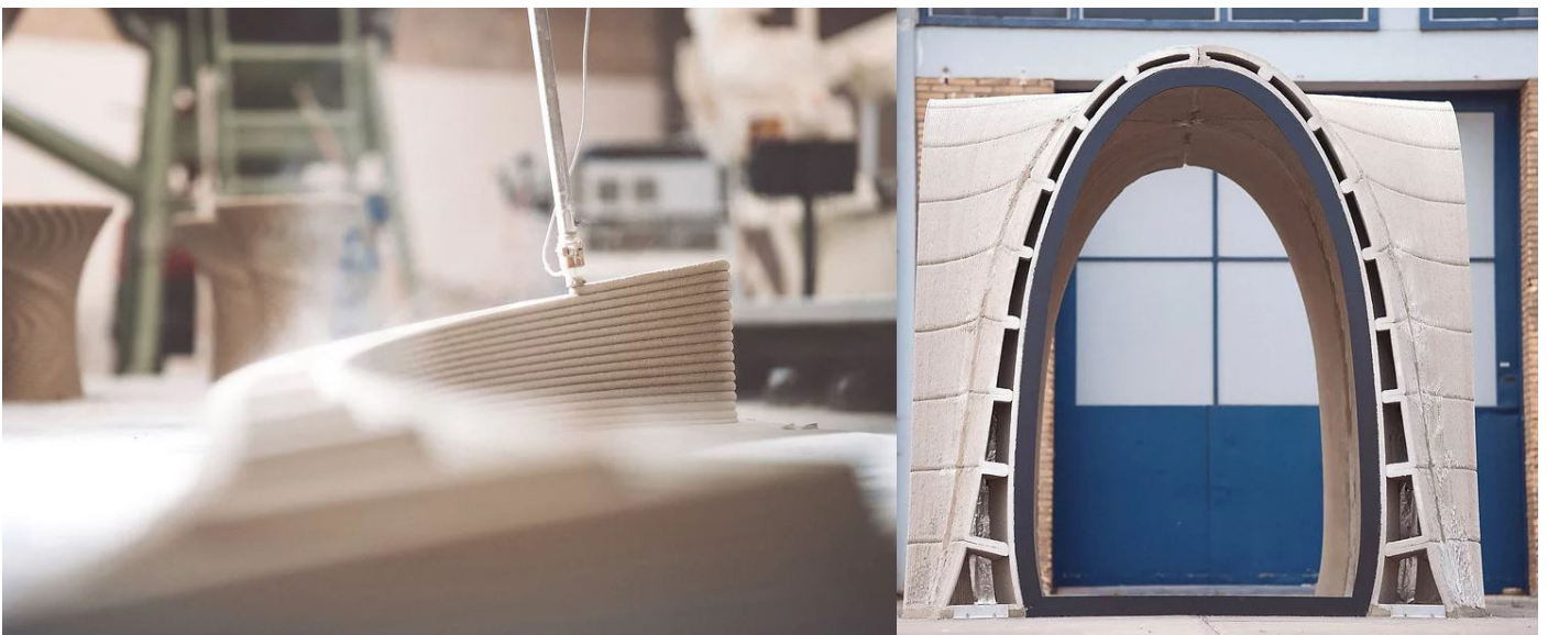
Fig. 3: Non-planar example of concrete printing. Source: [6]
