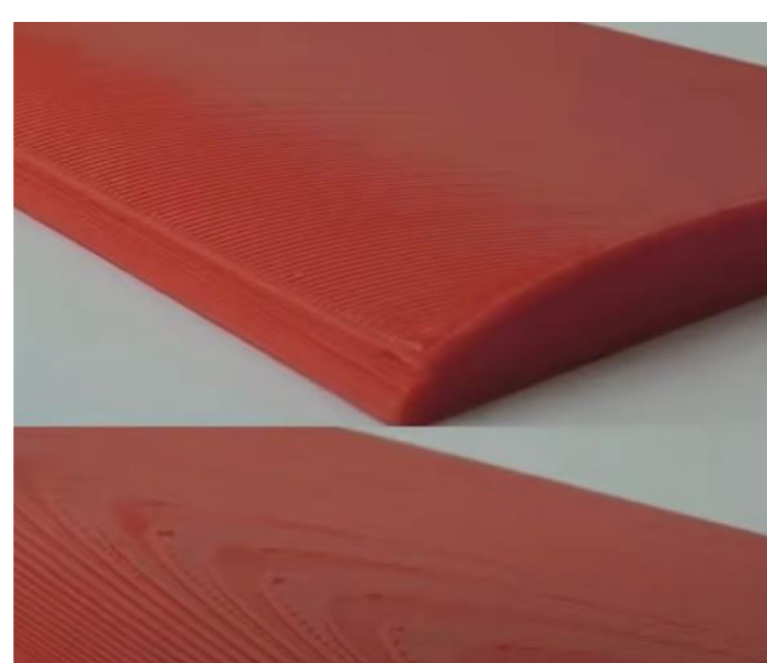
Fig. 4: Non-planar surface is smoother and more aerodynamic Source: [3]
