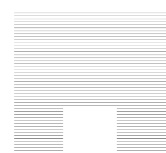
Fig. 9: Building openings for windows, doors, or plumbing can theoretically be printed non-planarly without any need of extra formwork. Vault-like layers could sustain pressure. However this approach needs testing.
