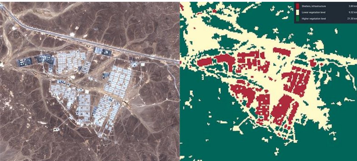
Satellite image of Azraq refugee camp from April 2017, three years after opening (left) and clustering algorithm result separating built structures from valley and mountainous terrain (right). The clustering result displays an increase in the built (shelter and infrastructure)
