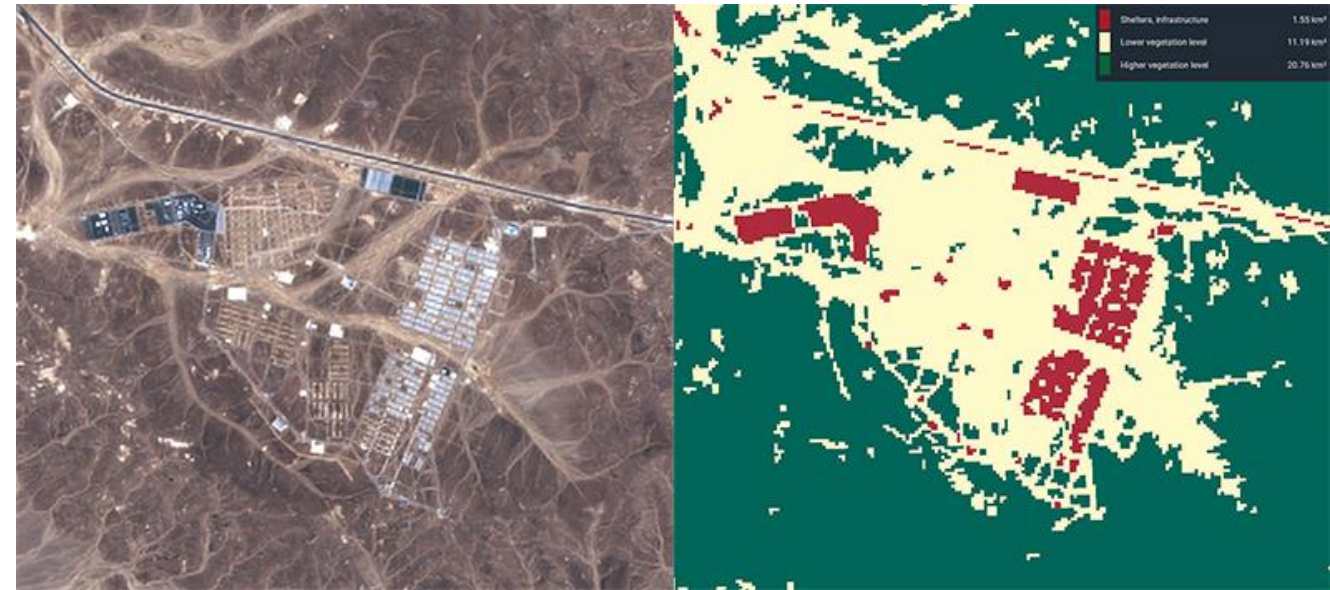
Satellite image of Azraq refugee camp from April 2014 when it was first opened (left) and clustering algorithm result separating built structures from valley and mountainous terrain (right).
